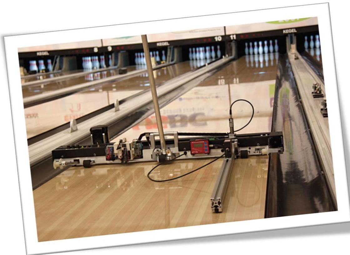
**Topography** is defined as the graphical representation of surface features indicating relative positions and elevations. It's a known fact that changes in topography adversely affect the ball path and ball motion (rate of energy depletion). When topographical features are randomly different on a bowling lane, so is ball motion which causes inconsistency.
