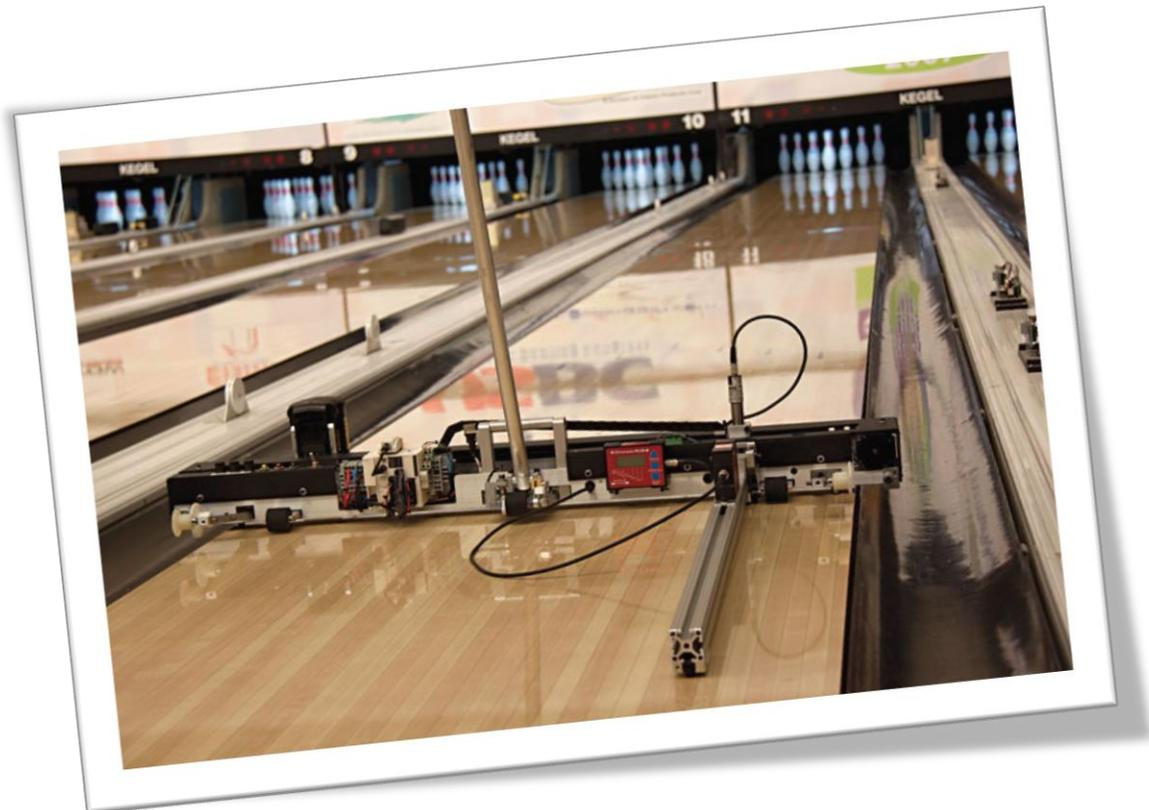
**Topography** is defined as the graphical representation of surface features indicating relative positions and elevations. It's a known fact that changes in topography adversely affect the ball path and ball motion (rate of energy depletion). When topographical features are randomly different on a bowling lane, so is ball motion.
